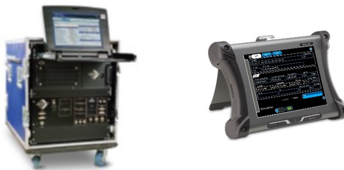
Figure 2-4 GPS Signal Simulator CAST-5000 [13] with 2 carriers – left, Cobham GPSG-1000 [14] with 1 carrier – right
