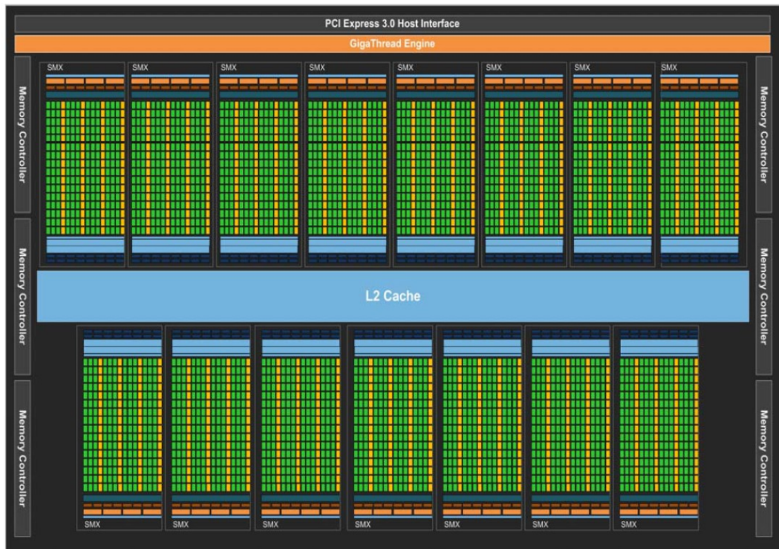
Figure 5-8 Architecture of Nvidia GPU GeForce GTX Titan Black with 15 SMXs, shared L2 cache and six memory controllers [67]
