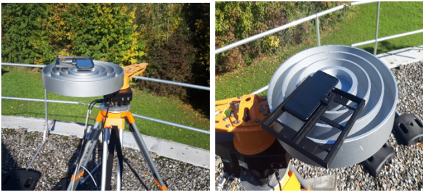
Fig. 20: Mi 8 choke-ring mounted on a rotating antenna
