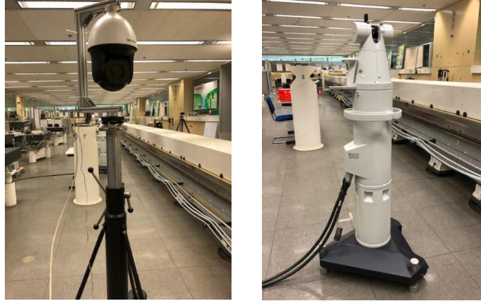
Figure 3. [Left] HD-IR camera. [Right] Laser interferometer
