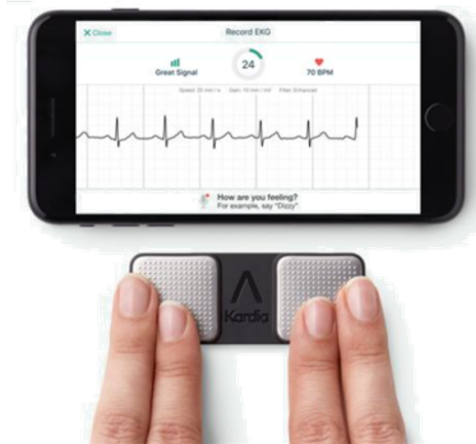
Figure 1. Recording of an electrocardiogram (ECG) with the KardiaMobile Device connected to the Kardia App. The single-lead ECG is recorded by laying the fingers on the electrodes of the KardiaMobile ECG device. A smartphone is connected to the device and records the ECG.
