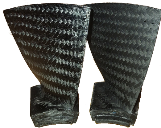
Figure 5. Initial (left) and final (right) versions of the composite blade.
