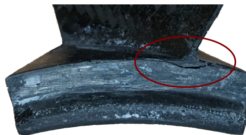
Figure 7. Typical damage pattern of delamination within the red circle at the blade’s backside transition from the root into the actual blade.
