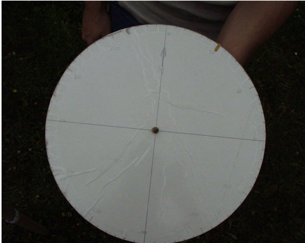
Figure 19: direction estimation device: disk with degree scale from below
