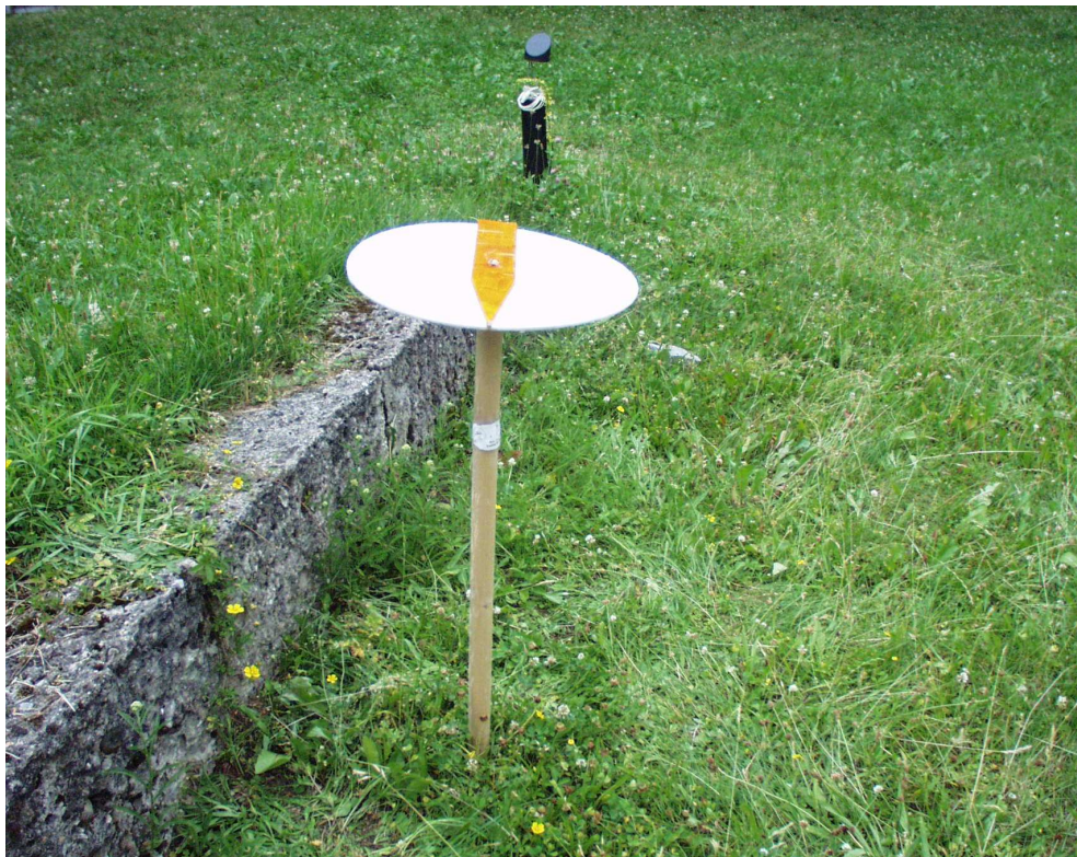
Figure 18: Direction estimation device: disk equipped with an arrow to indicate the chosen direction
