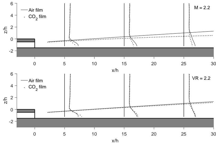
Figure 5: Comparison of blowing ratio (upper part) and velocity ratio (lower part).
