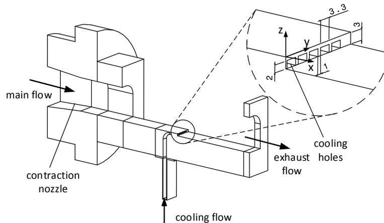
Figure 1: Test section model (coordinate system is indicated).
