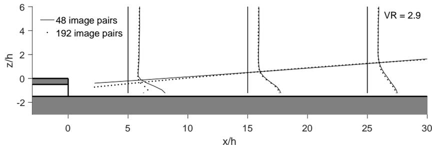
Figure 4: Boundary layer and velocity profiles for air cooling film - 48 image pairs vs 192 image pairs.
