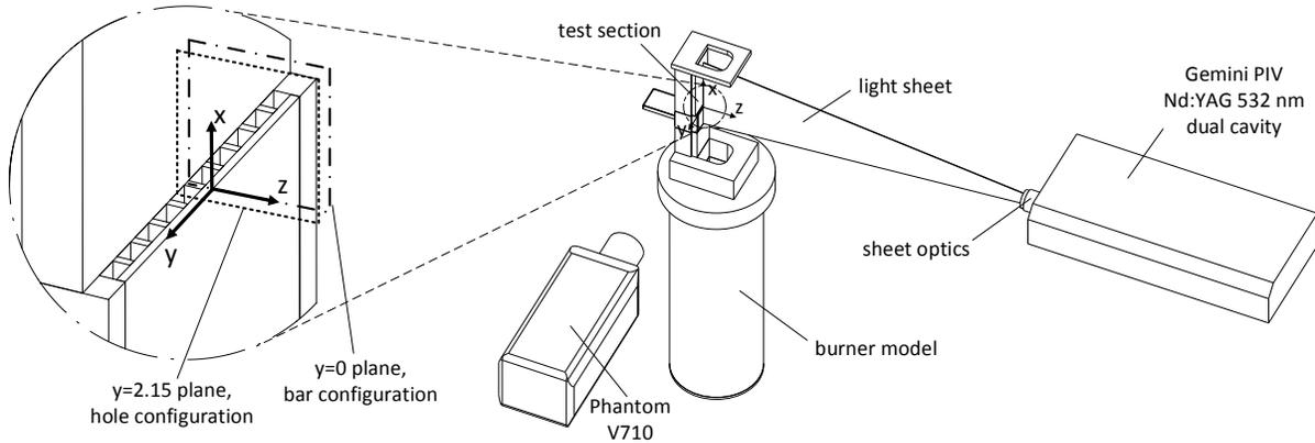
Figure 2: Experimental setup and laser sheet positions.
