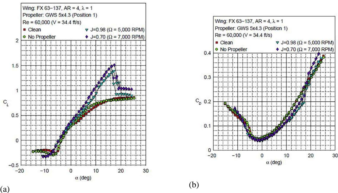
(a) Figure 2: Effect of propeller advance ratio on the lift and drag curve of the wing at  $Re = 60000$  (Ananda et al., 2013).
