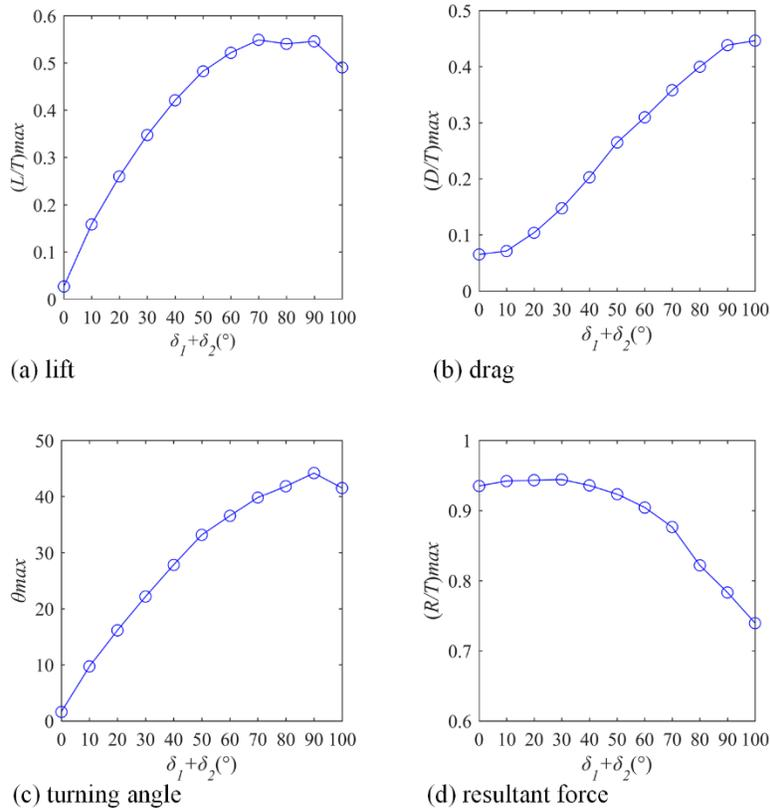
Figure 4 The aerodynamic performance of multi-element wing under propeller slipstream.
