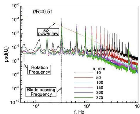
Figure 1: Power spectra of the axial velocity fluctuations at  $r/R = 0.51$  for different  $x$  positions (Mukund et al., 2016).
