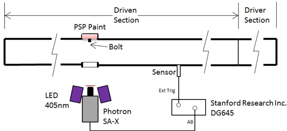
Figure1 A sketch of system arrangement
