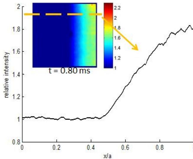
Figure5 Leading edge of shock wave at  $t = 0.80\text{ms}$
