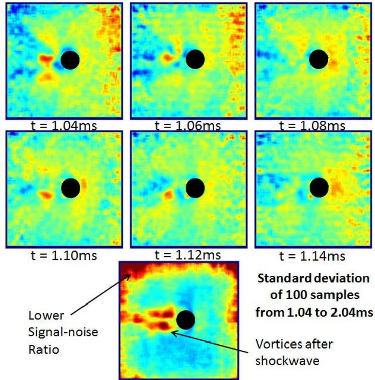
Figure6 Relative intensity fluctuation of PSP and standard deviation of 100 samples
