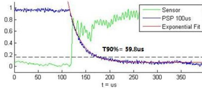
Figure4 Relative intensity ( $Ir^{-1}$ ) curve of PSP paint
