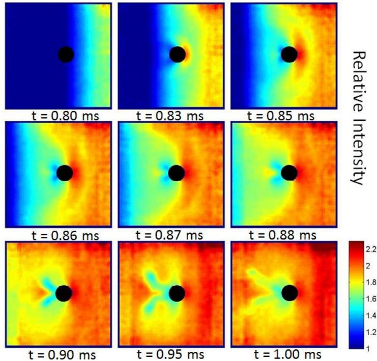
Figure 2 PSP results when shock wave crashes the bolt
