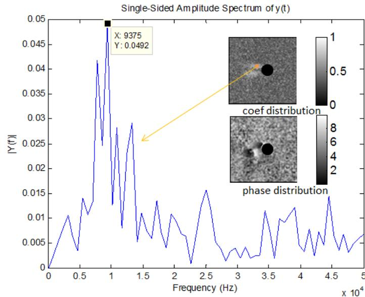
Figure7 FFT plot of single point, correlation and phase distribution
