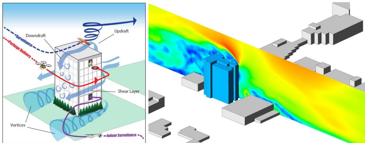
Figure 1 Possible flight path scenarios around a building (LHS) and a CFD simulation of wind around a nominally cuboid building in an urban environment (RHS), from Mohamed et. al. (2015).
