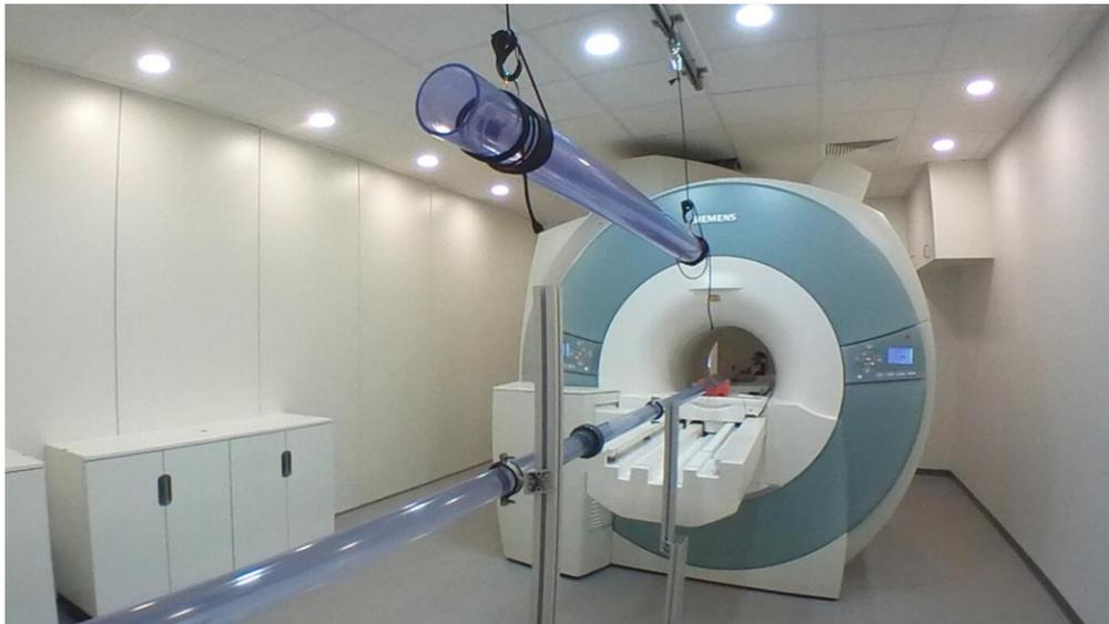
Figure 1: Picture of the MRI flow lab showing the MRI scanner and a flow circuit installation.
