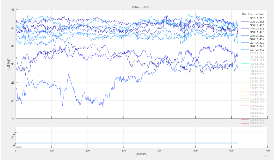
Figure 13: SNR plot for the static retransmission scenario
