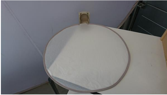
Fig. 11 The SDSS module with an unfolded/deployed sail.
