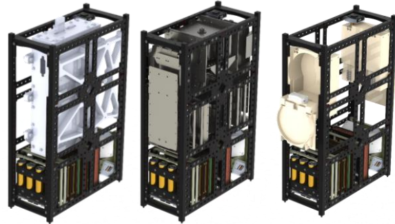
Fig. 6 Render of the Tesser PMD module prototype accommodating the three removal subsystems: The Solid propulsion (to the left), the EDT (in the centre) and the drag sail (to the right).
