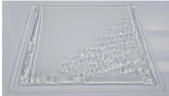
Figure 5.7: Failed reproduction of a previously successful print after some time without operating the L320 printer.
