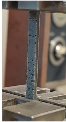
Figure 6.6: Estane specimen with tearing on the outer surface.
