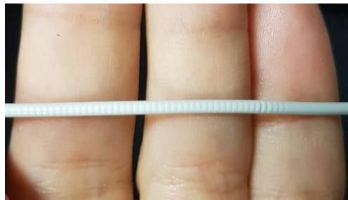
Figure 6.2: Indentation marks in the Arnitel filament from the extrusion process.
