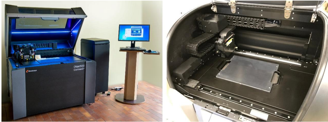
Figure 5.3: Objet500 Connex (left) and Agilista-3000 (right) 3D printer series [courtesy of WIWeB].
