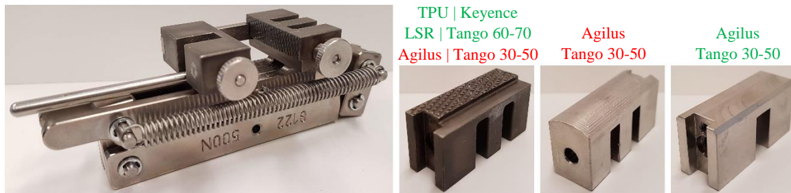
Figure 5.9: Pincer grip and the three types of clamping surface attempts (successful in green, unsuccessful in red).
