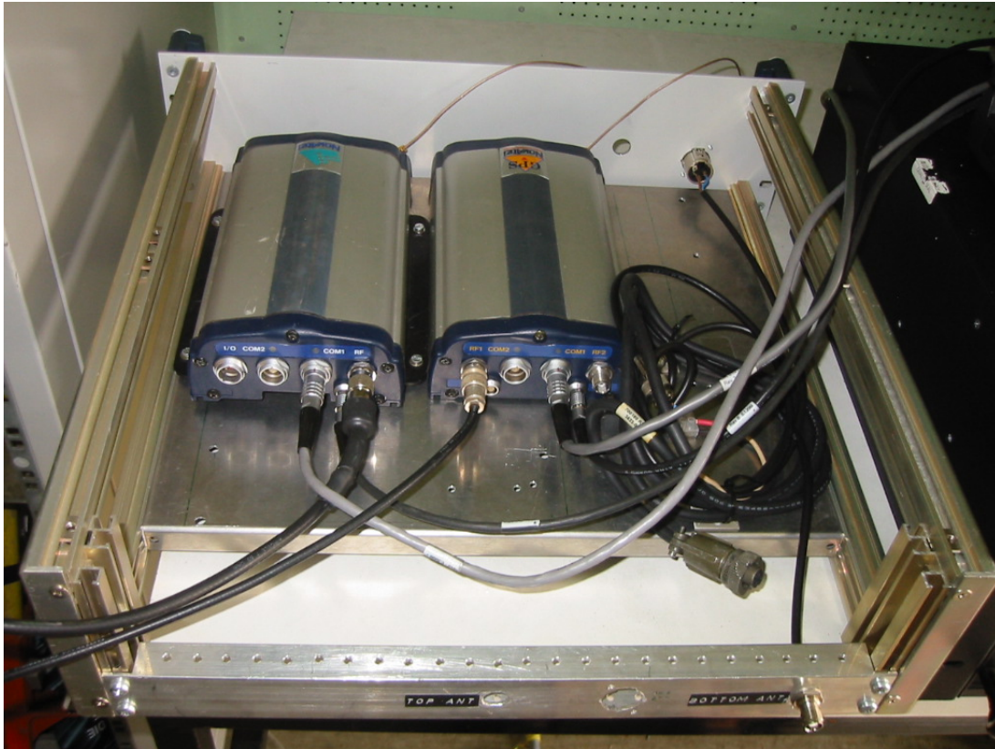
Figure 3-4: Modified NovAtel OEM3 Propak II L1 navigation receivers
