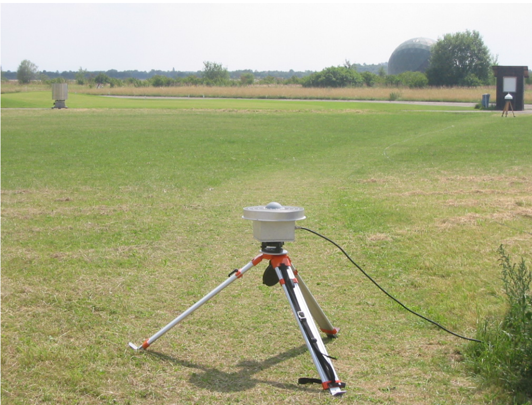
Figure 3-3: NovAtel 501 antenna with choke ring for APL signal transmitting
