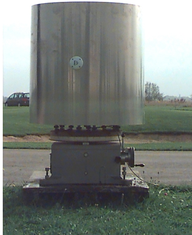
Figure 3-1: Aluminium cylinder on a precision turntable
