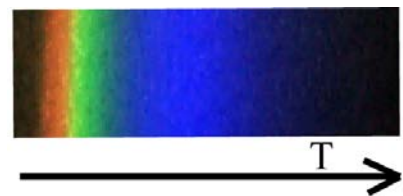
Figure A.2: Colour transition of the reflected light as function of the temperature
