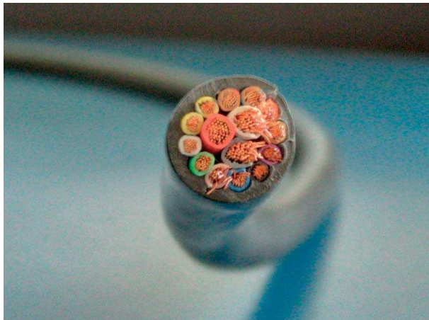
Fig. 7.1: Real multicable consisting of fifteen single cables.
