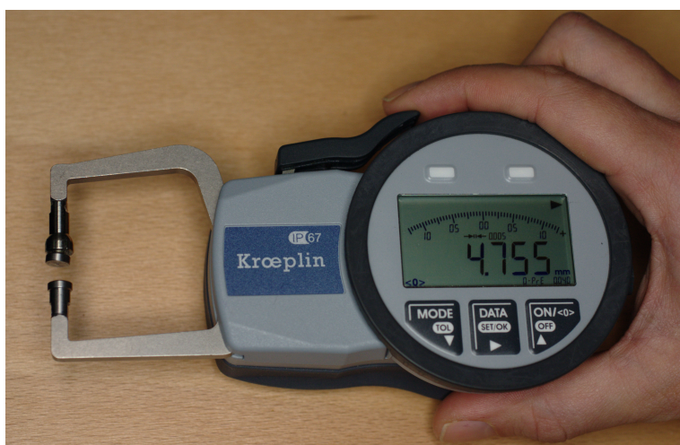
Figure 6.3: Measuring gauge for ear thickness determination (C1X079, Kröplin GmbH).
