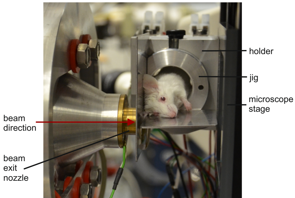
(b) The jig is placed in the heatable holder mounted to the stage of the microscope. The hole in the steel plate is positioned directly in front of the beam exit nozzle.
