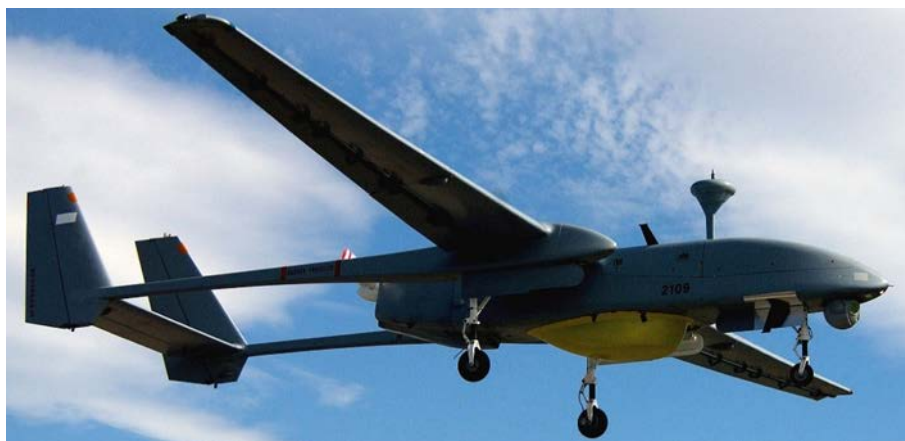
Figure 1-1: Unmanned aerial reconnaissance vehicle IAI Heron. The yellow fairing hides a synthetic aperture radar (SAR). Under the nose, the optical reconnaissance system is located. (Source: USAF)
