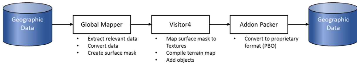
Figure 4-15: Toolchain to create VBS terrain databases.
