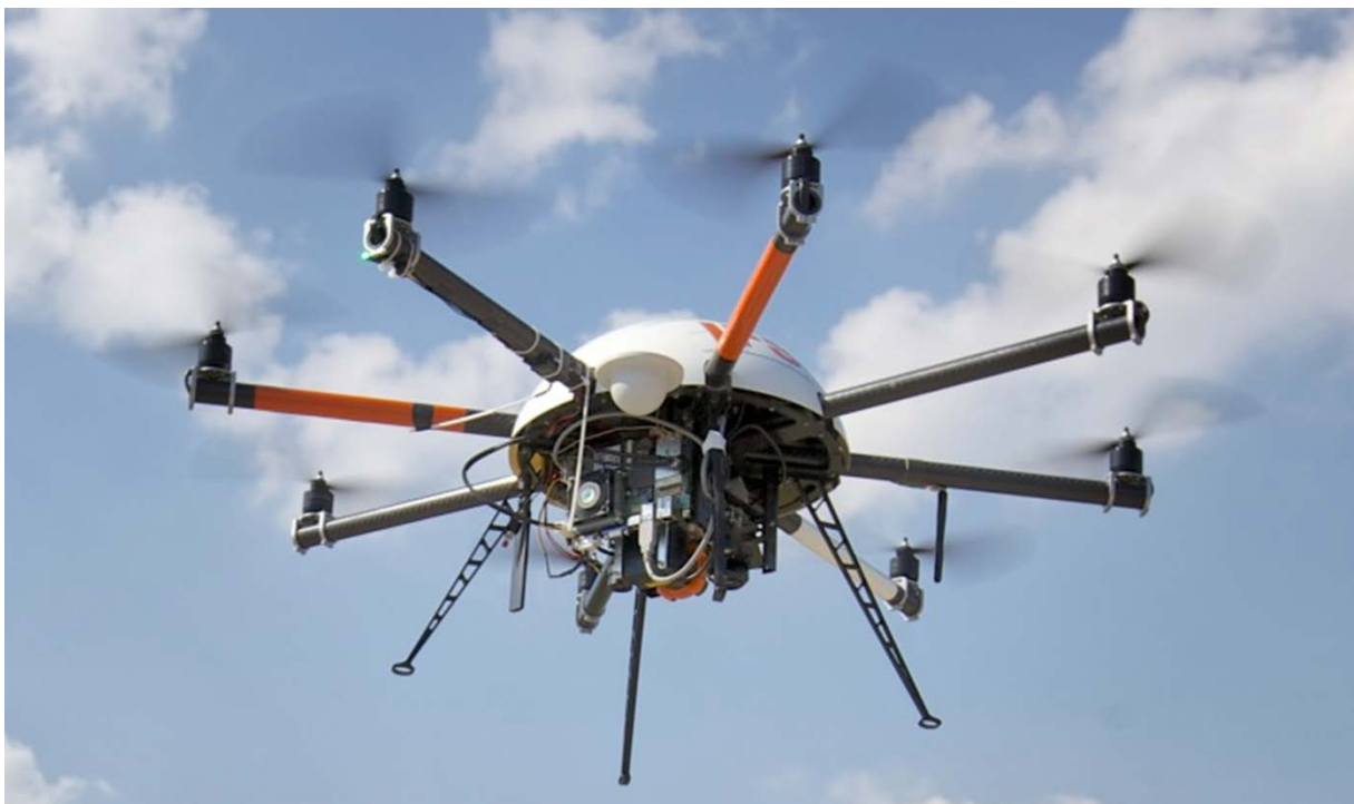
Figure 4-5: The unmanned Aerial Vehicle Octo XL used in the experiments for this thesis. In this image, a fully equipped payload can be seen (Russ, Schmitt, Hellert, & Stuetz, 2013).
