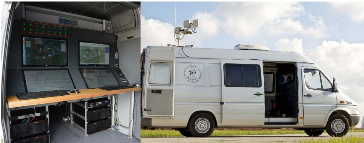
Figure 4-3: Left: The interior (left) and exterior (right) of the deployed ground control station. Note the antenna array located on the roof.
