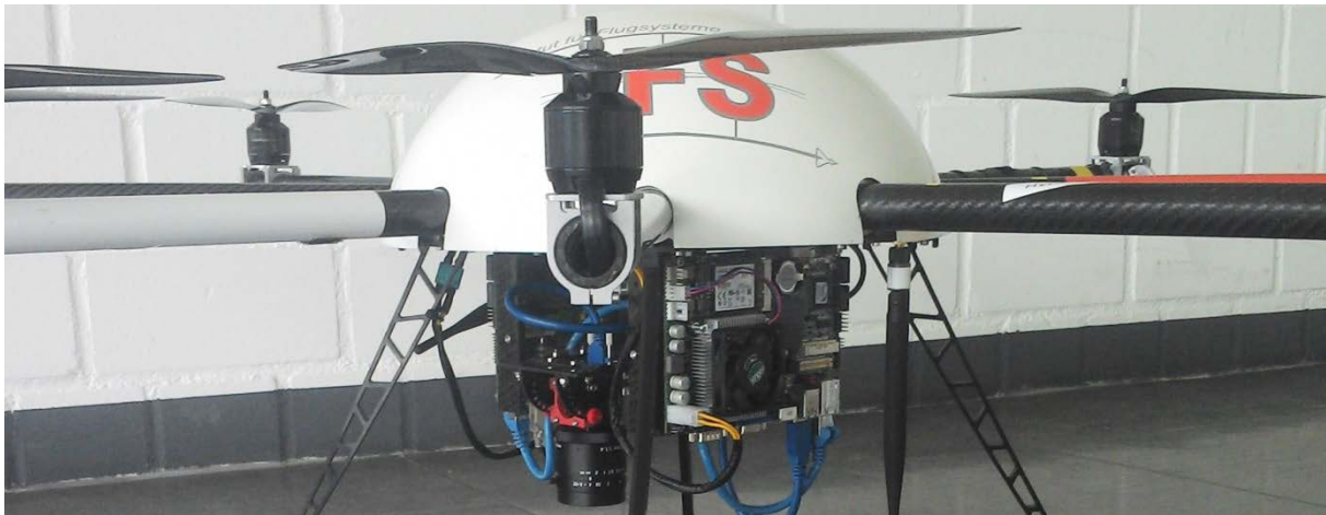
Figure 4-7: Experimental mission payload system as used for the test flights of this thesis.
