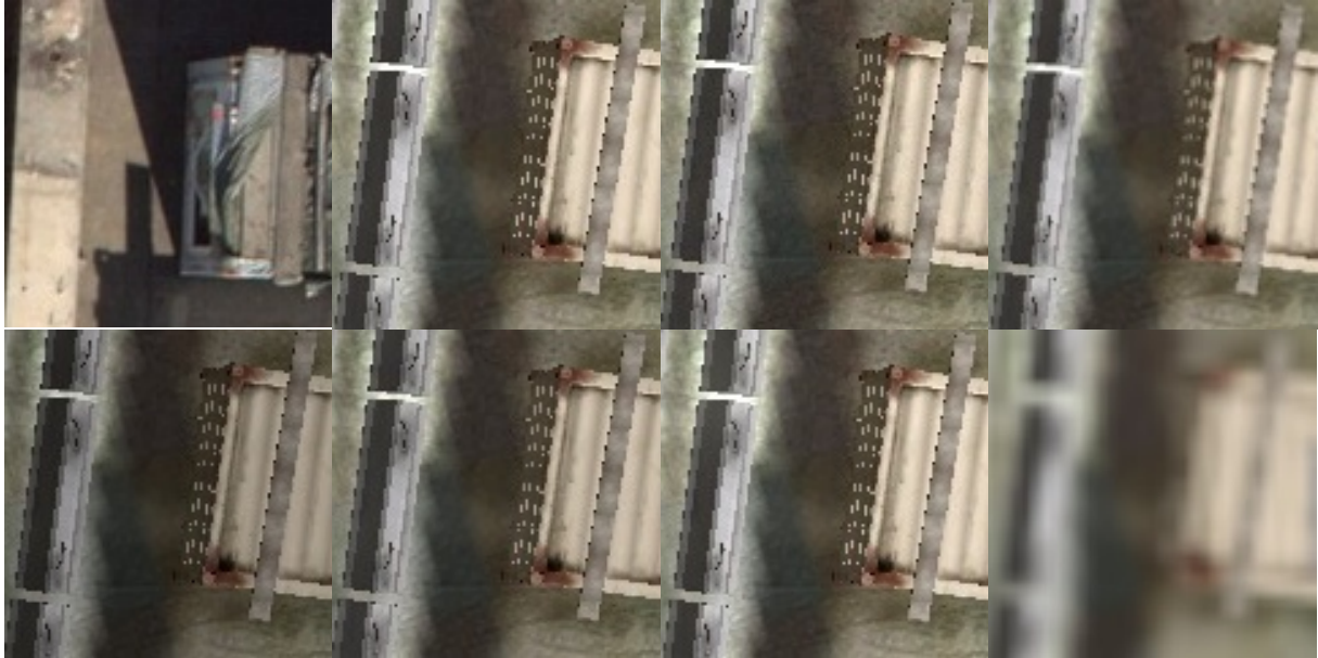
Figure 5-18: Configuration examples of set Camera Model on a snippet of image 35 of scene concrete . Upper left to lower right: photo , baseline , noise , distortion , aperture , HDR , bloom and blur .
