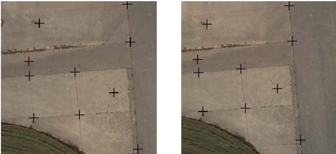
Figure 5-3: Image pair example (Frame 7869, left; Frame 7884, right) with annotated ground truth (black crosshairs).
