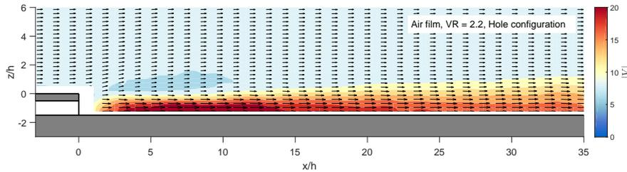
Figure 3: Contour plot air film,  $VR = 2.2$ .
