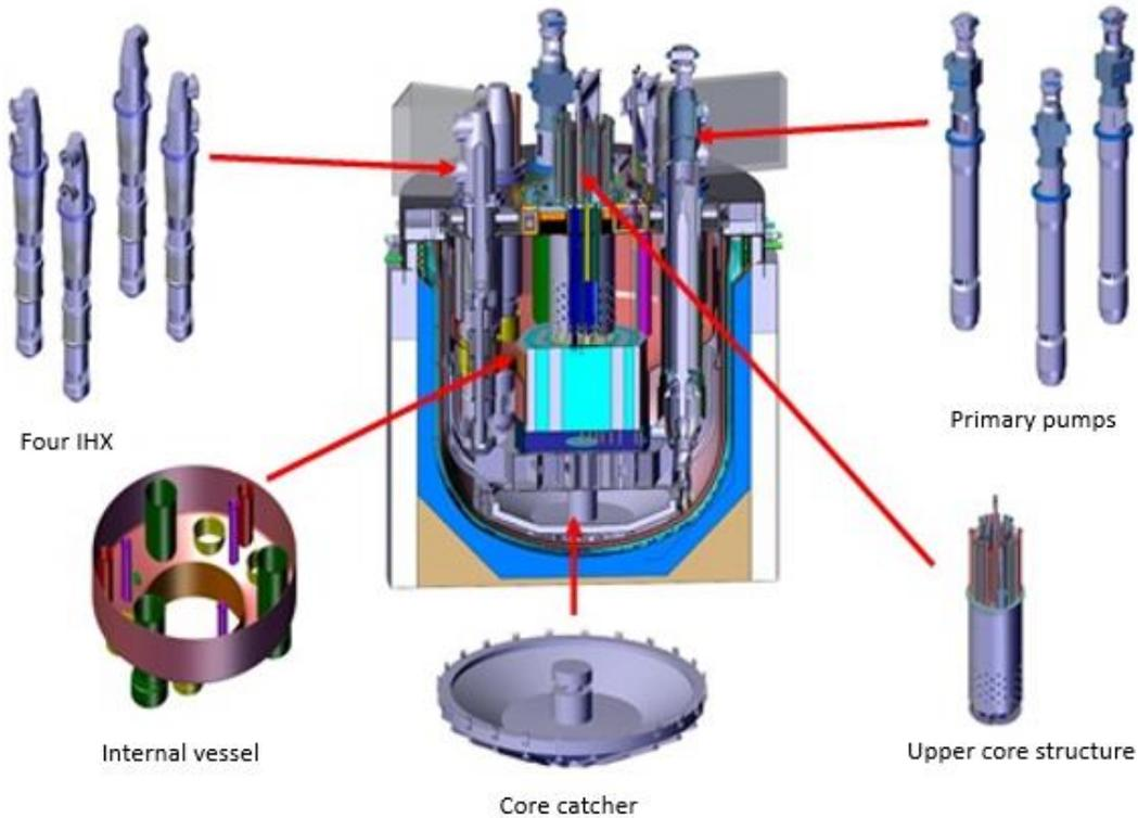
Figure 1: A cut view of ASTRID primary circuit
