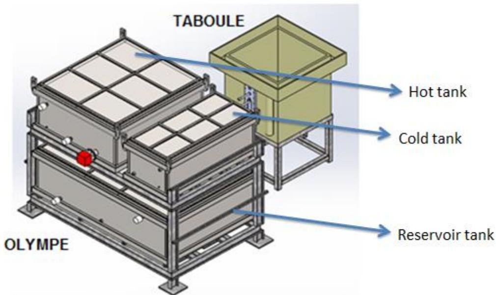
Figure 7: The two jet flow experimental facility
