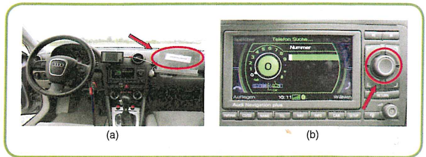
FIG 2 Secondary task and HMI of the test vehicle. (a) Position of the 25-digit number. (b) Rotate-and-press controller for operation of the speller function.
