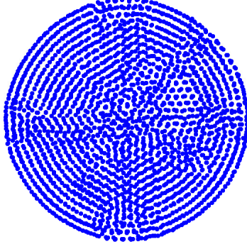
Figure 5.2: Low-gravity validation: Surface tension: Converged particle distribution at time t = 0.2 s, showing a slice of thickness \Delta y = [-0.1, +0.1] mm (i.e. a layer of 4 particles in y -direction) through the fluid
