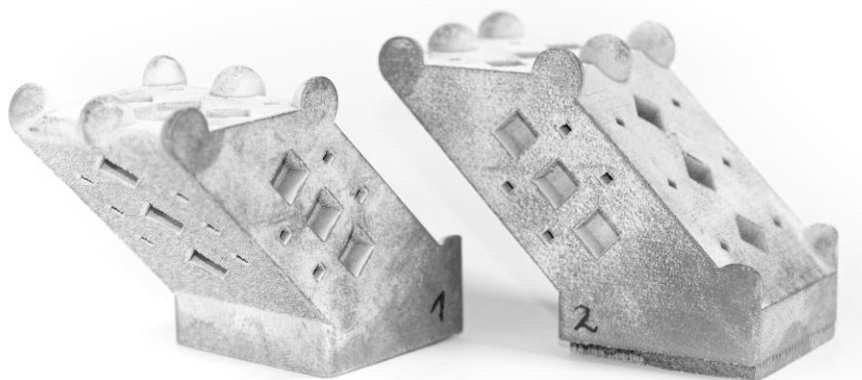
Figure 3. The artefact manufactured by different L-PBF systems
