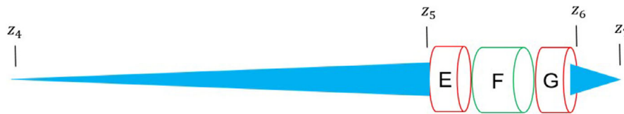
FIG. 11. Sketch of the focusing system consisting of a quadrupole triplet and two drift lengths after the linear accelerator for the buncher configuration U_b = 35 \text{ kV} and longitudinal focus at the input to linac structure. At the maximum beam size within the lenses, 90% of the particles fit into a circular aperture with a diameter of 44 mm. [Color figure can be viewed at wileyonlinelibrary.com]
