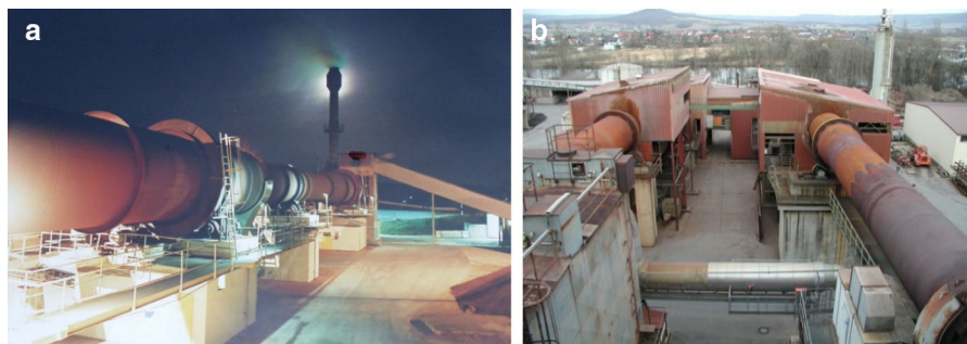
Fig. 11 a Two-part rotary kiln (double body) with preheater and expansion shafts (Source: Liapor GmbH & Co. KG) and b Expanded clay kilns successfully tested for the productions of calcined clay (Pautzfeld plant, Germany (b) [41]).
