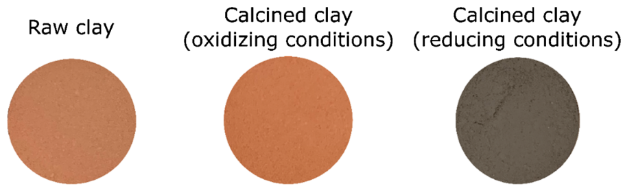
Fig. 10 Colour of raw and calcined iron-oxide containing (3.8 wt%) kaolinic clay under oxidising conditions and reducing conditions. Adapted from Refs. [22, 129]
