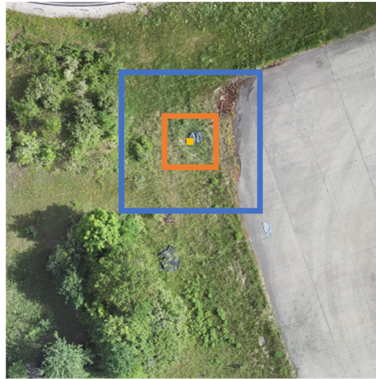
Figure 5. Dual window neighborhood principle for anomaly detection. For the pixel under test (marked yellow), only pixels that are inside the blue window but outside the orange area are considered for estimating its anomaly score.
