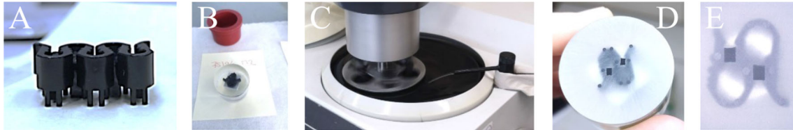
Fig. 3 Preparation of samples for microhardness indentation
