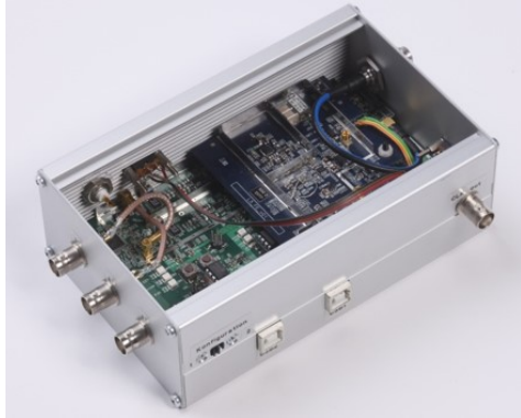
(a) TriBand USB2.0 Front-end from 2006
