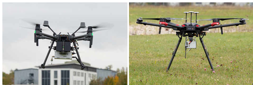
Figure 2. Experimental multicopter platforms with integrated MMT device.
