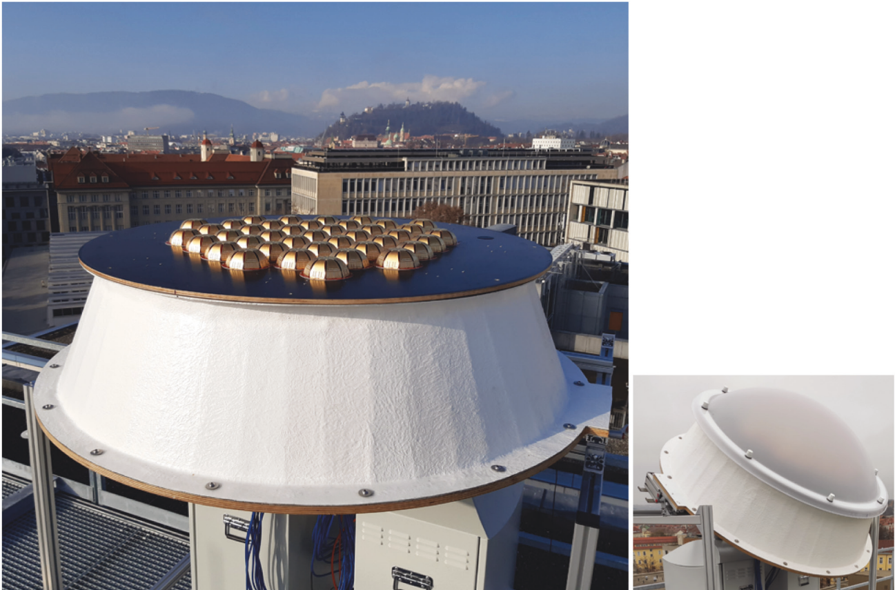
FIGURE 3 Antenna array opened (left) and tilted with a radome (right)
