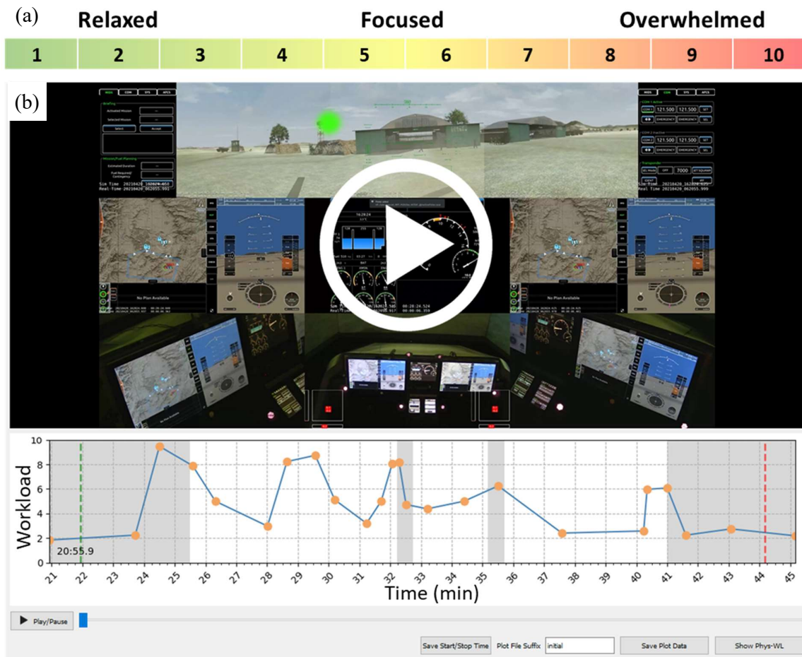
Fig. 4.4 Tool developed to gather a participant's subjective mental workload post-flight. Subfigure (a) shows the Likert scale used by the participants to evaluate their own subjective mental workload on a scale from 1 to 10. Subfigure (b) shows the graphical user interface (GUI) used by the experimenter and participant to collect the subject's subjective mental workload over the duration of a recently-concluded simulated helicopter mission. Views internal and external to the cockpit are provided along with the pilot's gaze location (green icon) providing rich contextual information to aid in subjectively assessing mental workload. The data in the plot is edited by the experimenter as directed by the participant to reflect the participant's subjective mental workload over the course of the simulated mission.
