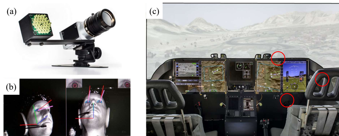
Fig. 2.7 Various elements of the eye-tracking system. Sub-figure (a) shows the IR transmitter (left) and camera (right) used in the Smart Eye Pro eye tracking system. Sub-figure (b) shows the real-time pupil and iris detection used in the SmartEye Pro system. Sub-figure (c) is a photograph of the helicopter simulator with the three eye-tracking cameras on the right cockpit circled in red.
