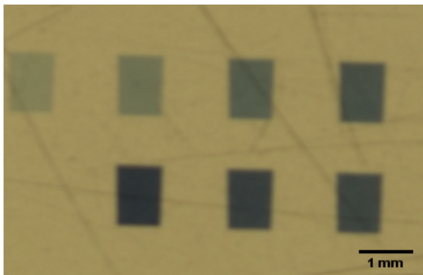
Figure 2.7: The EBT-3 gafchromic film irradiated for calibration by using the calibrated photomultiplier as detector. The doses 0.5 Gy, 1 Gy, 2 Gy, 3 Gy, 4 Gy, 5 Gy, and 7 Gy were irradiated in fields of 1.12 mm x 0.8 mm size.
