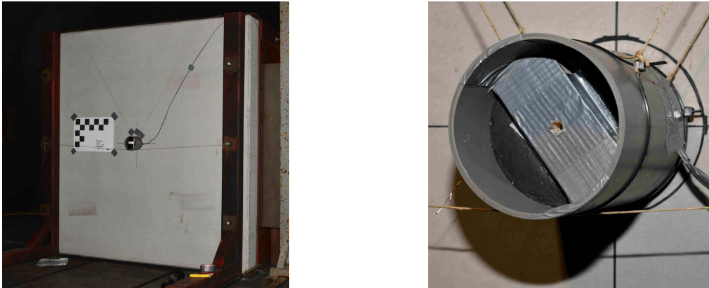
Figure 4.1.: Experimental setup from detonation side (left) and detail explosive (right)
