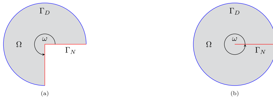
Fig. 1. Circular sectors \Omega with angle \omega and the corresponding boundaries. (a) \omega = \frac{3}{2}\pi . (b) \omega = 2\pi .
