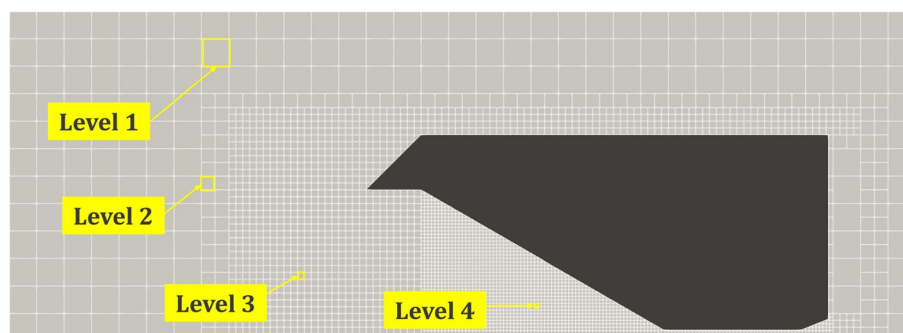
Fig. 7 Grid detail: multi-level refinement of the cartesian grid, after the grid adaptation
