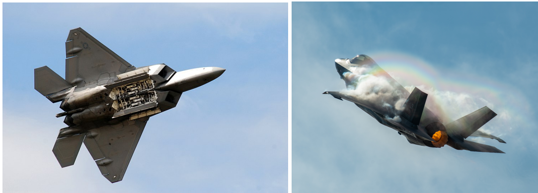
FIGURE 1.1: F-22 Raptor shows its weapon bay (left) [6] and a vortex forms around the body of the F35 aircraft (right) [7]
