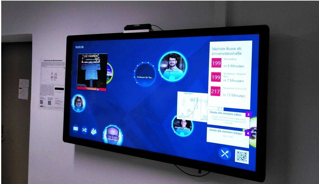
Figure 22: Setup of display in 41/400 20G – with the ZED 2 camera on top of the screen – fixed with a 3D printed mount
