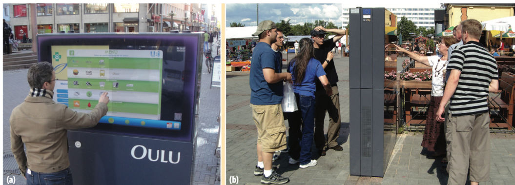
Figure 33: Outdoor UBI hotspots (a) along a walkway, where a user is interacting with version 2 of the UBI portal and (b) in the market area of downtown Oulu. Each outdoor hotspot is a double-sided display accessible 24/7 (Ojala et al. 2012)
