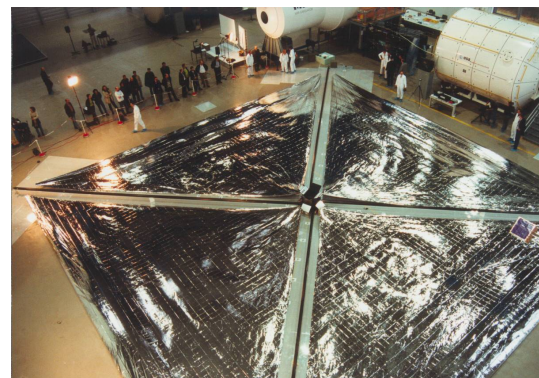
2.3.2: Deployed (20\text{ m})^2 solar sail at DLR
