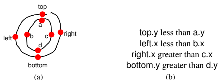
Figure 5.4: Example of an unconnected shape and its constraints. The origin is in the upper left corner.
