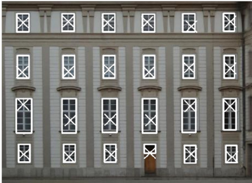
Figure 2.10: Facade interpretation (MAYER and REZNIK 2007) – hypotheses of window centers (crosses) and extracted windows (boxes) after MCMC search.
