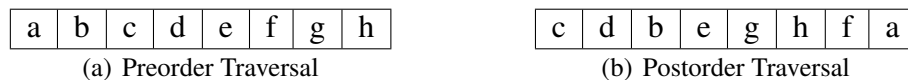
Figure 3.2: Tree traversal algorithms align the tree onto a sequence. This example shows two possible traversals of the tree displayed in Figure 3.1(a).
