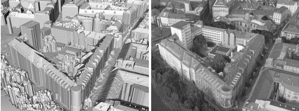
Figure 1.3.: Shaded and textured 2.5D model from Graz. The model results from SGM disparity maps on aerial images. (HIRSCHMÜLLER 2008) © 2008 IEEE
