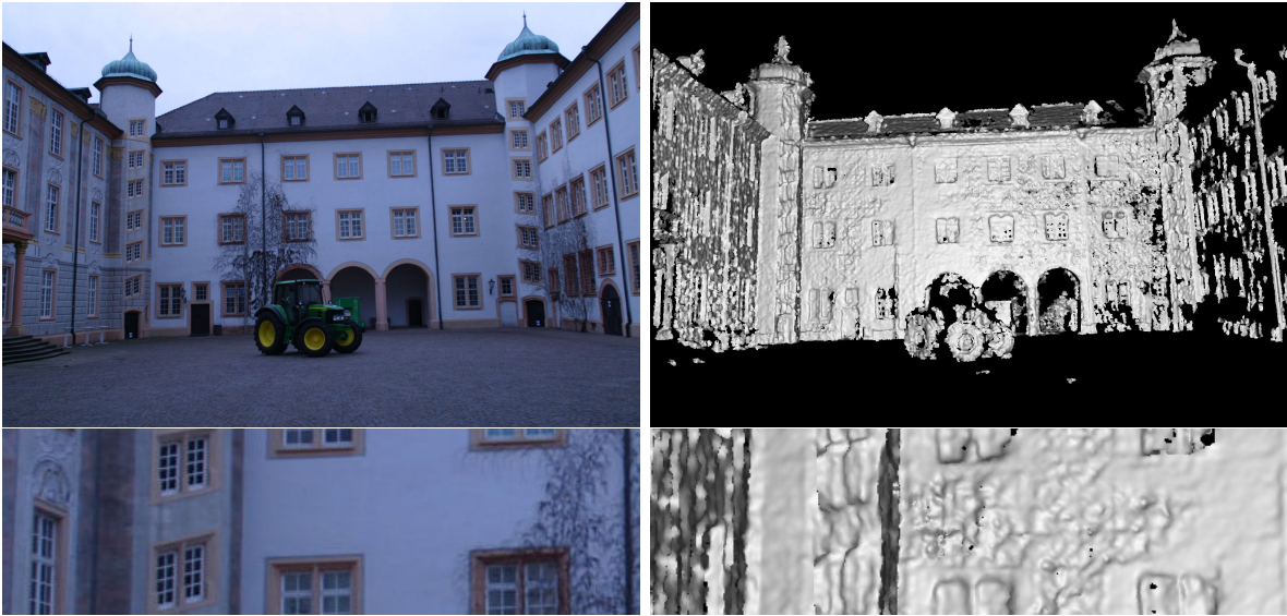
Figure 5.7.: Left: (Zoomed) image of the Ettligen30 sequence (STRECHA et al. 2008). Right: Coded image that shows the slant to the surfaces estimated from the depth map that considers 48 neighboring values. The coding ranges from 0^\circ (white) to 90^\circ (black). In this image, the slant provides a reasonable impression of the reconstruction quality of the surfaces. Untextured and non-fronto-parallel regions are mostly not precisely reconstructed.
