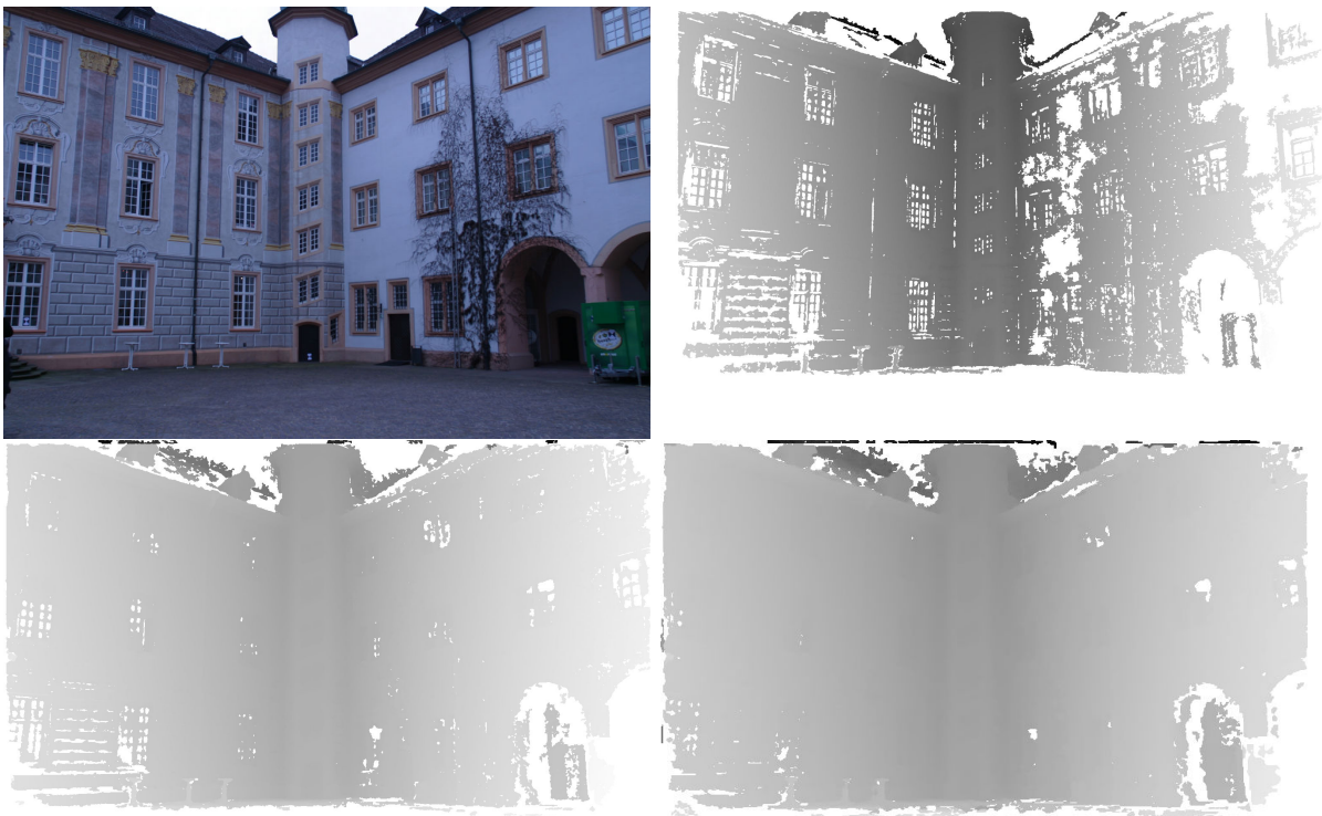
Figure 6.6.: Three disparity maps obtained by images downsampled with factor 1, 2 and 4. In the upper left the original image from the Ettligen30 sequence is shown. Low resolution image lead to higher densities and can even have better accuracy.
