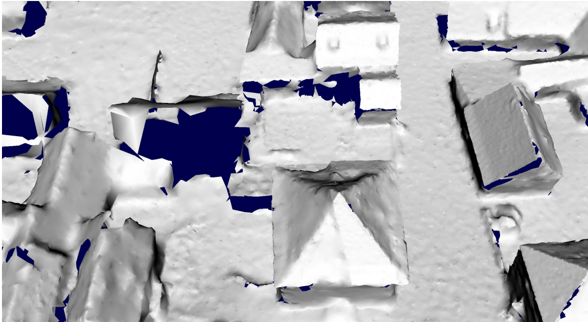
Figure 7.20.: This image shows the same part of the model shown in Fig. 7.4. The registration error was successfully used for regularization because the roof is not hard-edged any more. In addition, the ground is smoothly reconstructed. Because of the large number of images, the resolution is much lower, creating a high loss of accuracy.
