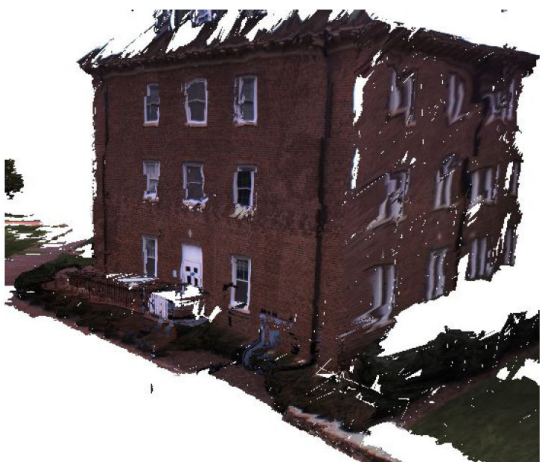
(c) Colored outdoor surface model from a building captured by a camera from the street. (MERRELL et al. 2007) © 2007 IEEE
