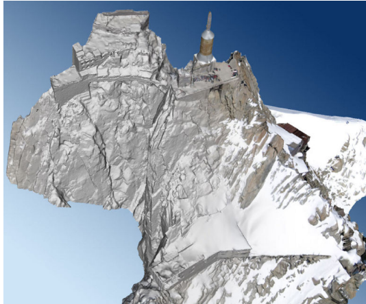
(a) Colored and shaded surface with fine details obtained by complex refinement. (VU et al. 2012) © 2012 IEEE
